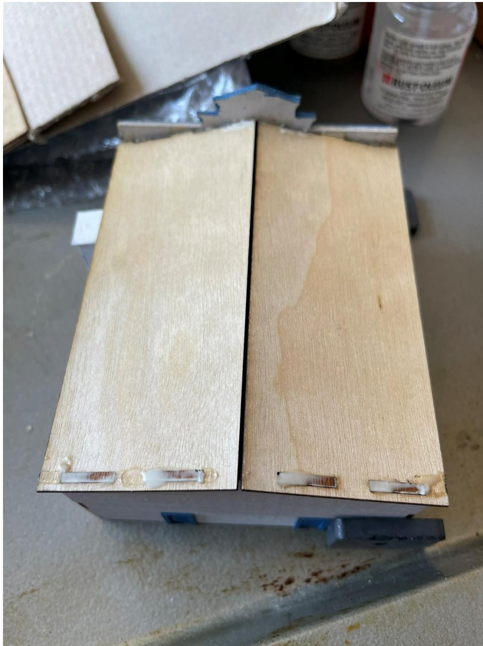
After this assembly had dried for a day, I inserted the interior wall and reinforced all the interior corner joints with strips of wood from the leftovers of the laser-cut sheets. Hopefully this will keep this fragile structure solid for many years...
