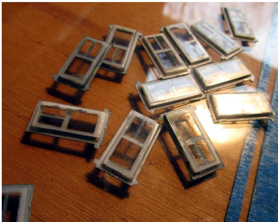
Canopy glue, which I'm using for almost everything else in this model, also works well for making window panes if they are small. It will dry completely clear. In this case I didn't feel like cutting little circles to fit.
